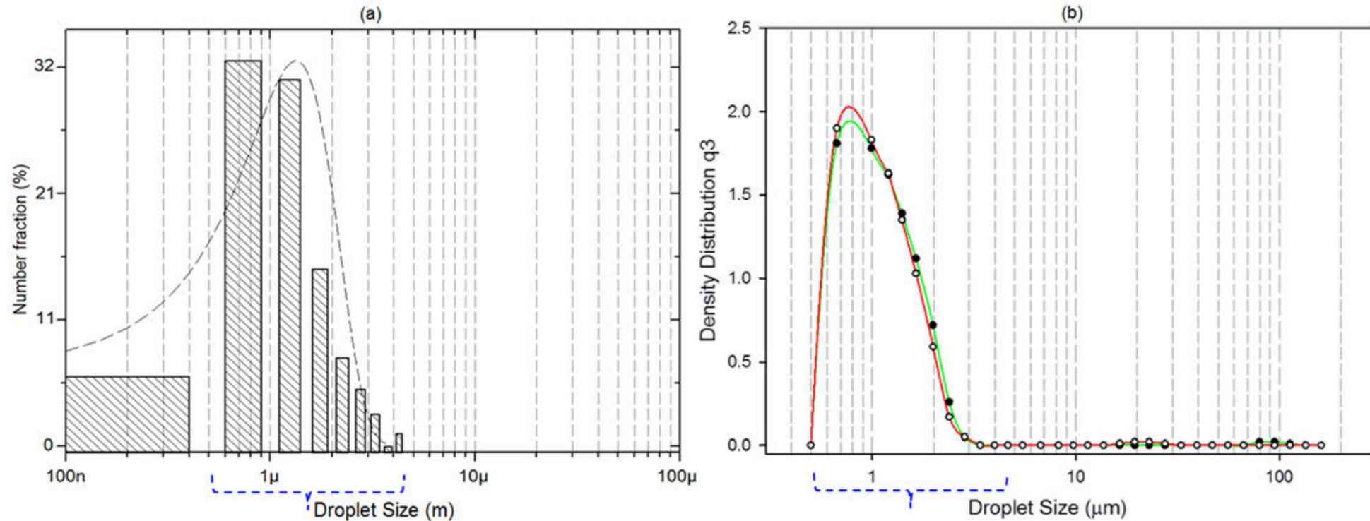
Comparison of (a) fluid-droplet model and (b) experimental observations of size distribution of droplets using HMDSO precursor droplets at flow rate =  $100 \text{ mL min}^{-1}$  and gas flow rate =  $5 \text{ L min}^{-1}$ ,  $f = 20 \text{ kHz}$  and  $V_0 = -13.5 \text{ kV}$ .
