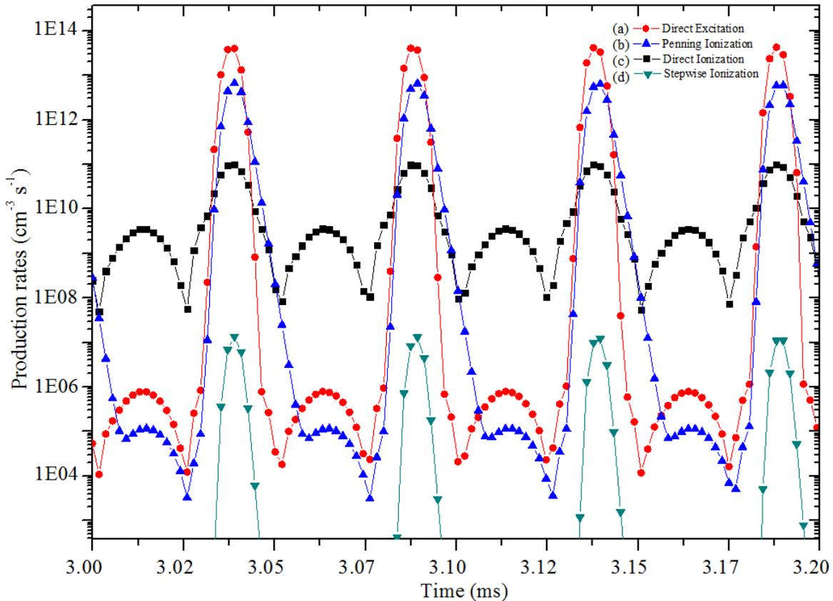
Penning ionization has been recognized as dominant as compared other ionization processes.
