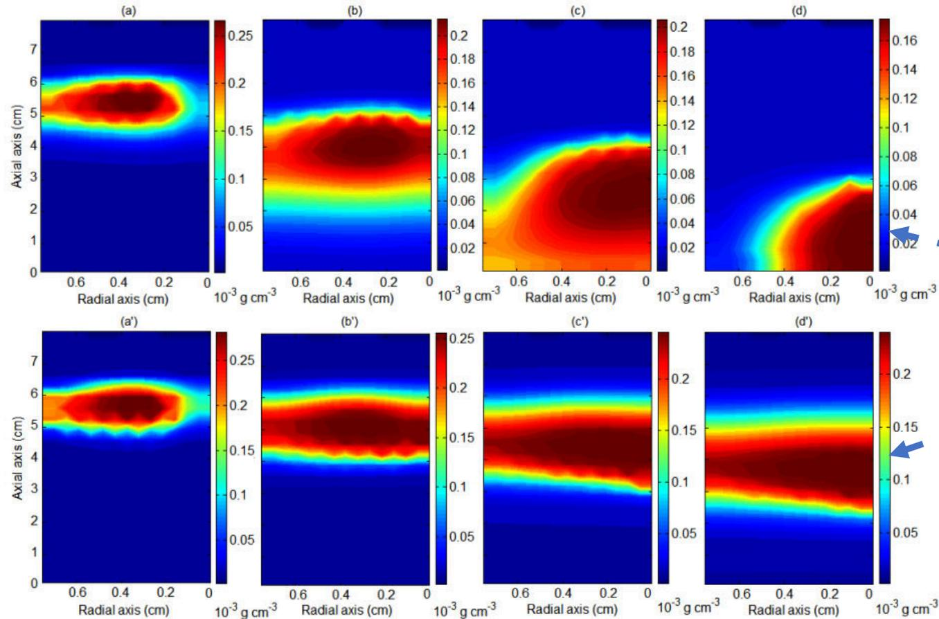
Download pull and evaporation of droplets is more stronger in the case of APP at the top row as compared to the He-N<sub>2</sub> gas mixture at the bottom row.
