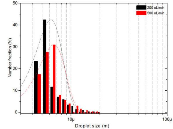
Droplet size distributions after 14 msec during downward flight of HMDSO droplets
