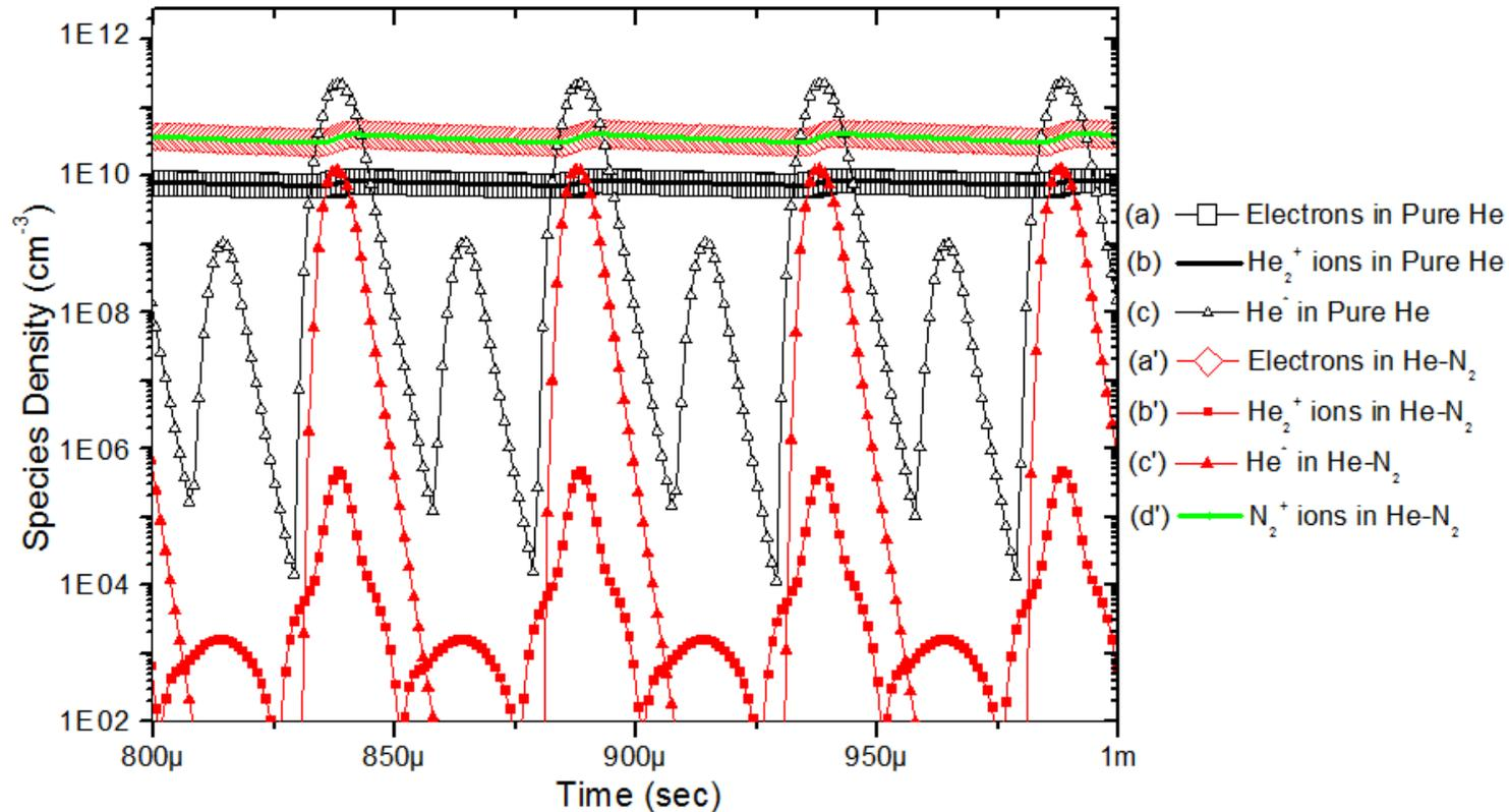
Comparison of line-averaged species density (electrons, He<sub>2</sub><sup>+</sup> ions, N<sub>2</sub><sup>+</sup> ions and He\*) in the pure Helium and He-N<sub>2</sub> gas mixtures using HMDSO droplets at precursor flow rate = 100 μL min<sup>-1</sup>, gas flow rate = 10 L min<sup>-1</sup>,  $f = 20$  kHz and  $V_0 = -13.5$  kV.
