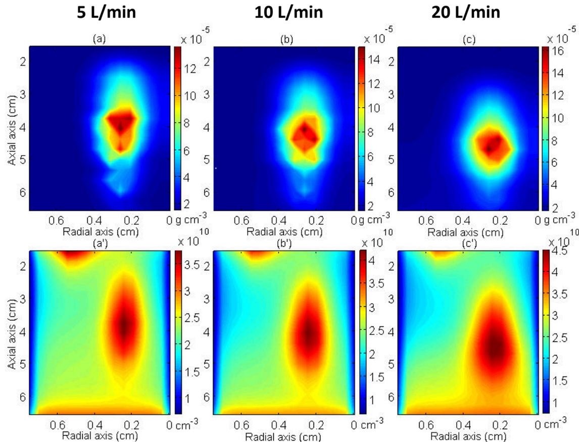
Variation in the vapour species density for different gas flow rates (5, 10 and 20 L min<sup>-1</sup>) at approximately 2 msec
